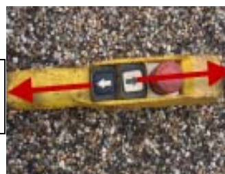
Wire rope inwards/up ramp Black Arrow
